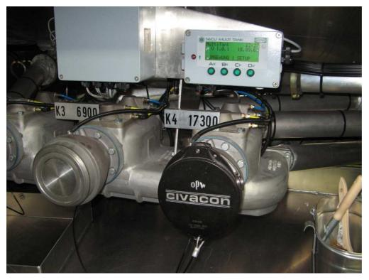
Practical example Installation of a SECU MultiTerm into a tank truck
